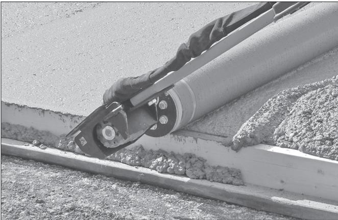
5. If necessary, handle may be moved to an offset position. Loosen knob (A), remove pins (B) and (C), move handle and handlebar assembly to offset position. Install pin (B) and tighten knob (A). Lower pin (C) will not be used when handle is in the offset position.
